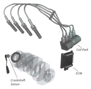
The crank-triggered, waste spark ignition system uses a crankshaft position sensor, coil pack, and available ECM to replace the distributor and coil used in conventional ignition systems, so servicing of distributor caps and rotors is eliminated. Crankshaft position is precisely determined directly from the crankshaft, resulting in improved spark accuracy. The OEM-established spark timing cannot be changed by the end user.
